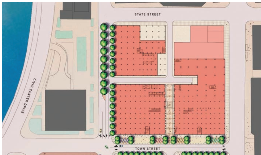
The Lazarus building fills an important part of Columbus' downtown and its history. To promote development to the south, the main entry was moved from High St. to Town St. The Galleria runs north/south from Town St. to the mid-block alley (approximately 185 ft.) at Chapel St. There is a two-story grade change from High St. to Front St. Site plan: courtesy of Schooley Caldwell Associates
